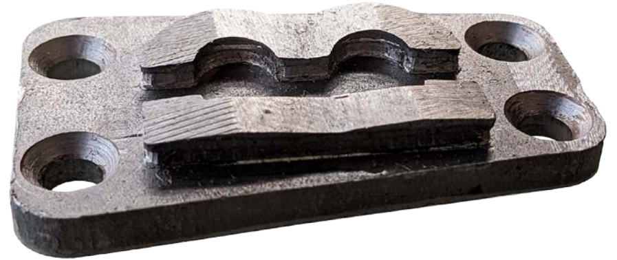
Punch of the letter B for a 1.75 inch Diagraph Jumbo.
